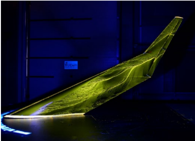
FIGURE 3: Large vortex structures appear at high angles of attack over the inner wing of the Flying V. 6
