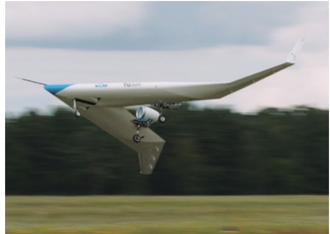
FIGURE 4: Flight control was experimentally verified using a 5%-scale flight-test demonstrator. Photo: Joep van Oppen for KLM and TU Delft
