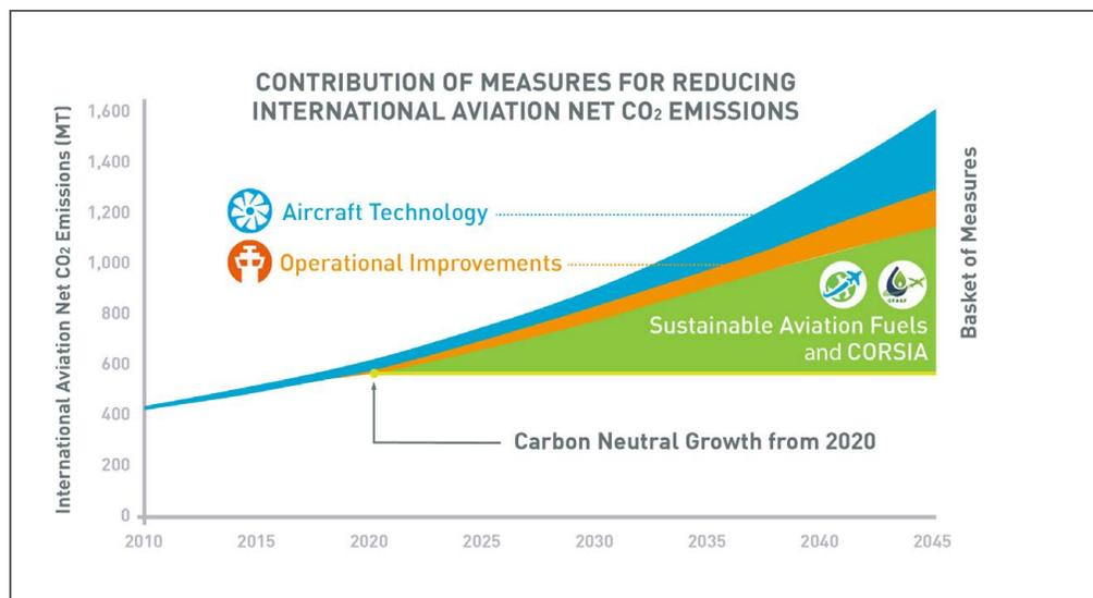
result, overall absolute emissions have increased as shown in Figure 1. The gains in energy intensity were achieved through better aircraft scheduling, higher passenger loads, and the commissioning of new and more efficient aircraft. Without these improvements, energy consumption in the aviation sector would have been 70 per cent higher in 2016 (IEA).
