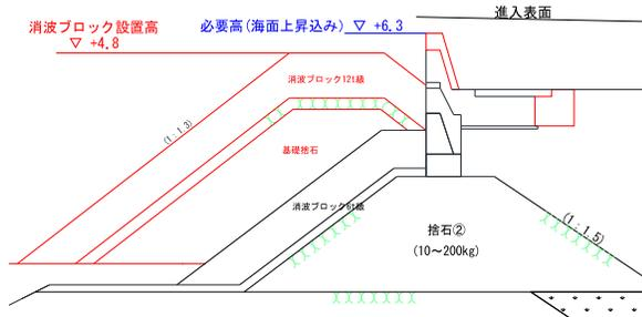
Below is the cross-section of the protective barrier with a raised protective seawall only.
