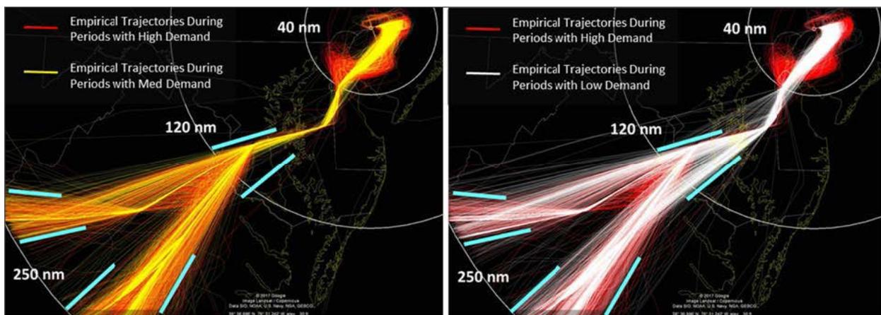
metering in the US. For instance, there is very little difference in actual trajectories during medium (yellow) and high (red) demand, resulting in a sea of orange with only a few red segments, indicating heavier vectoring and longer down-winds in high demand periods (see Figure 10). Such “predictability” of flown tracks is necessary for the existing metering algorithms to produce a feasible metering schedule. During low (blue) demand periods, evidence of shortcuts exists.
