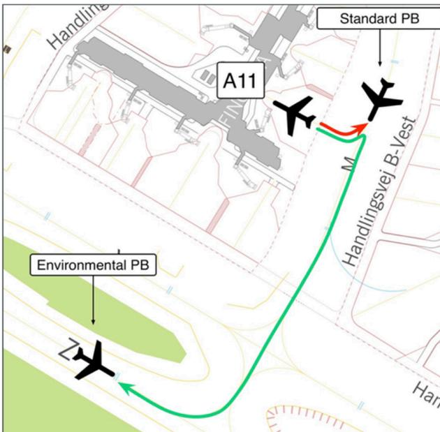
**Figure 4.** Illustration of the environmental push-back procedure.
