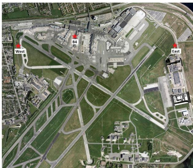
**Figure 1.** Overview of Copenhagen Airport. The red stars illustrate the locations of the airport's air quality monitoring stations: Station West (NO, NO<sub>2</sub>, PM<sub>2.5</sub> and UFP), Station East (NO, NO<sub>2</sub>, PM<sub>2.5</sub>) and the apron station, Station B4 (NO, NO<sub>2</sub> and UFP).
