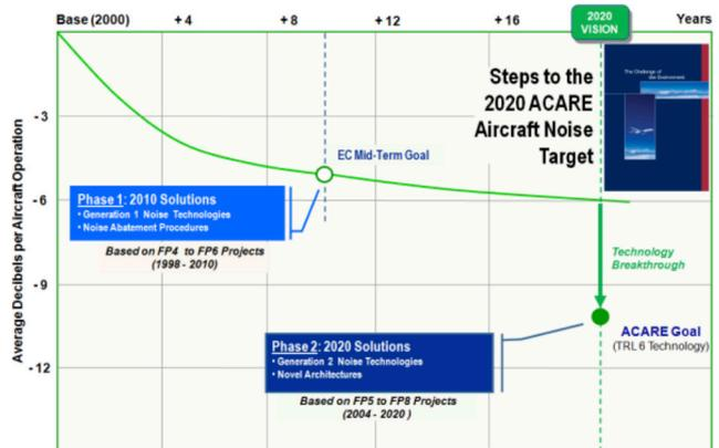
Figure 1. Steps to ACARE 2020 noise target.
