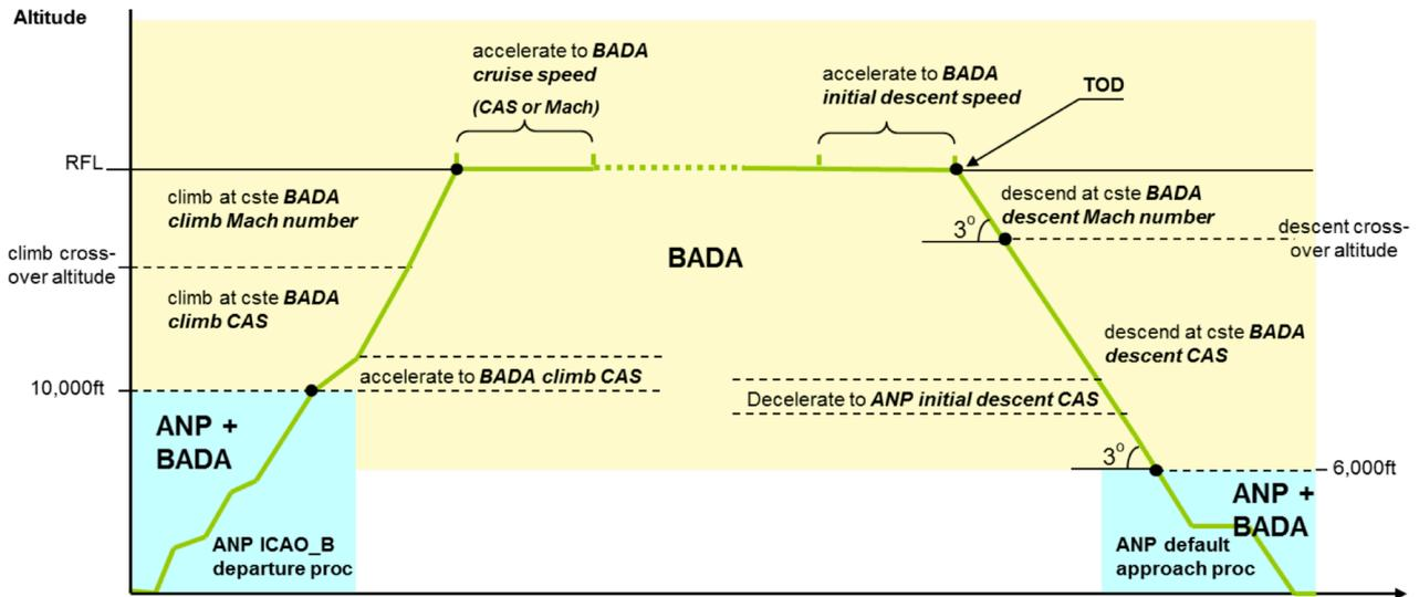
Figure 1. IMPACT full flight procedure used in CAEP<sup>1</sup>.
