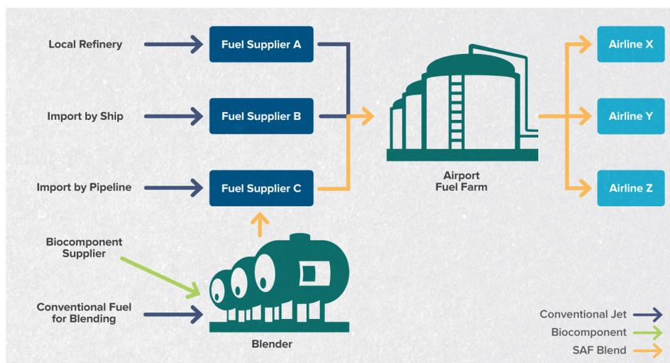
The fuel supply chain schematic illustrated above is based on the situation at a specific candidate airport. Supply chain modifications will vary on an airport-by-airport basis. Note that the blender can be a new or existing fuel supplier.
