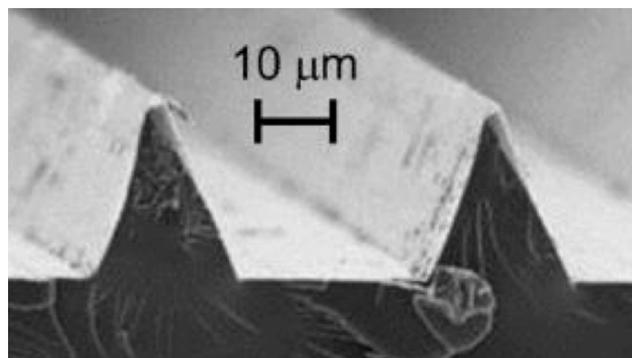
**Figure 1.** Microscopic Image of Surface With Riblet Shape<sup>1</sup>.
