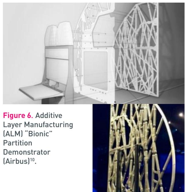
**Figure 6.** Additive Layer Manufacturing (ALM) “Bionic” Partition Demonstrator (Airbus)<sup>10</sup>.
