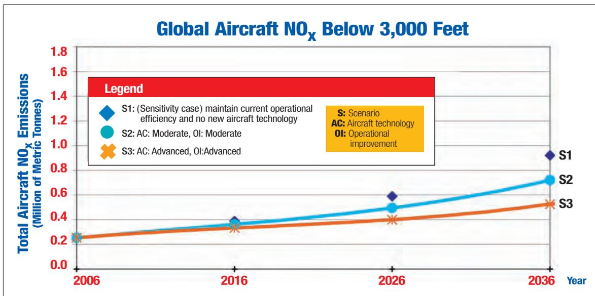
Figure 2: Total global aircraft NO<sub>x</sub> below 3,000 feet (915 Metres) AGL.
