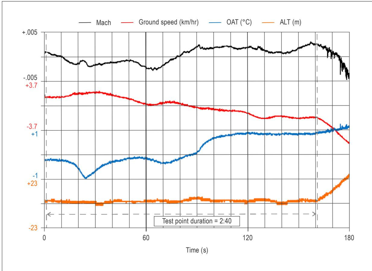
Figure 3-1. Flight test data time interval selection – Example 1
