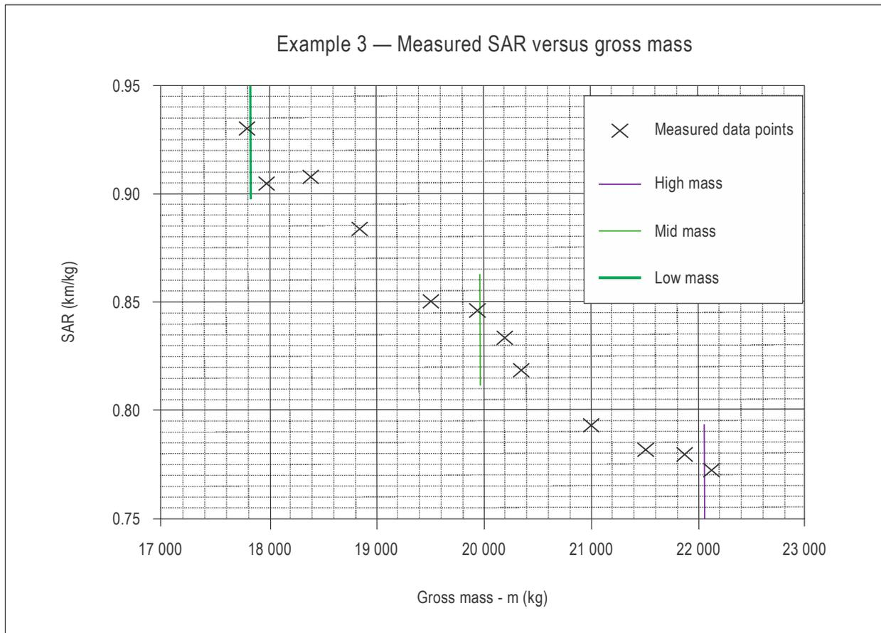
Figure 3-4. Measured SAR versus gross mass – Example 3
