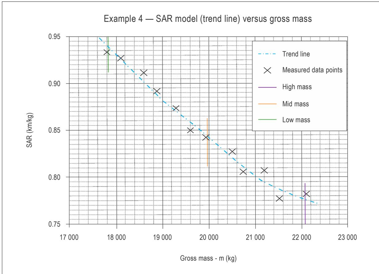
**Figure 3-8. SAR model (trend line) versus gross mass – Example 4**
