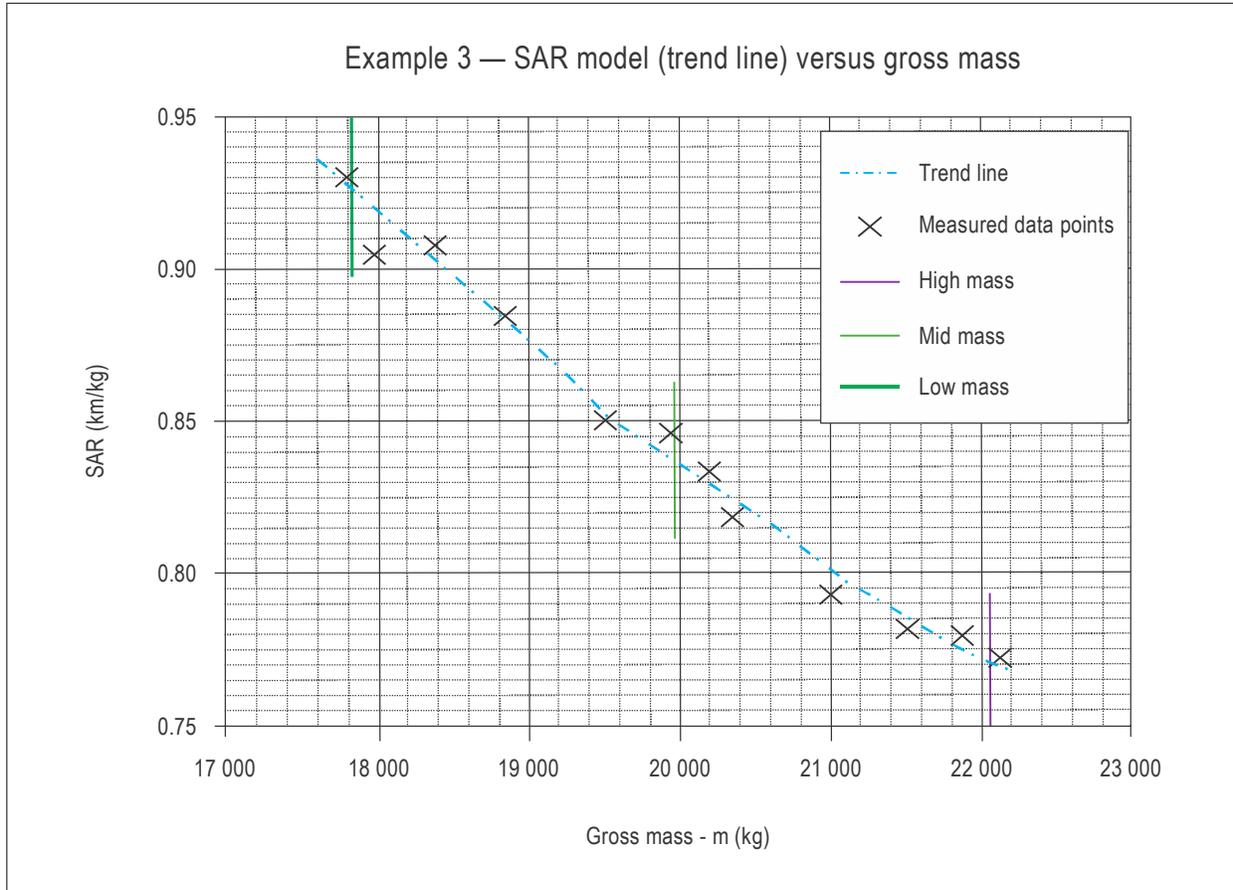
**Figure 3-5. SAR model (trend line) versus gross mass – Example 3**
