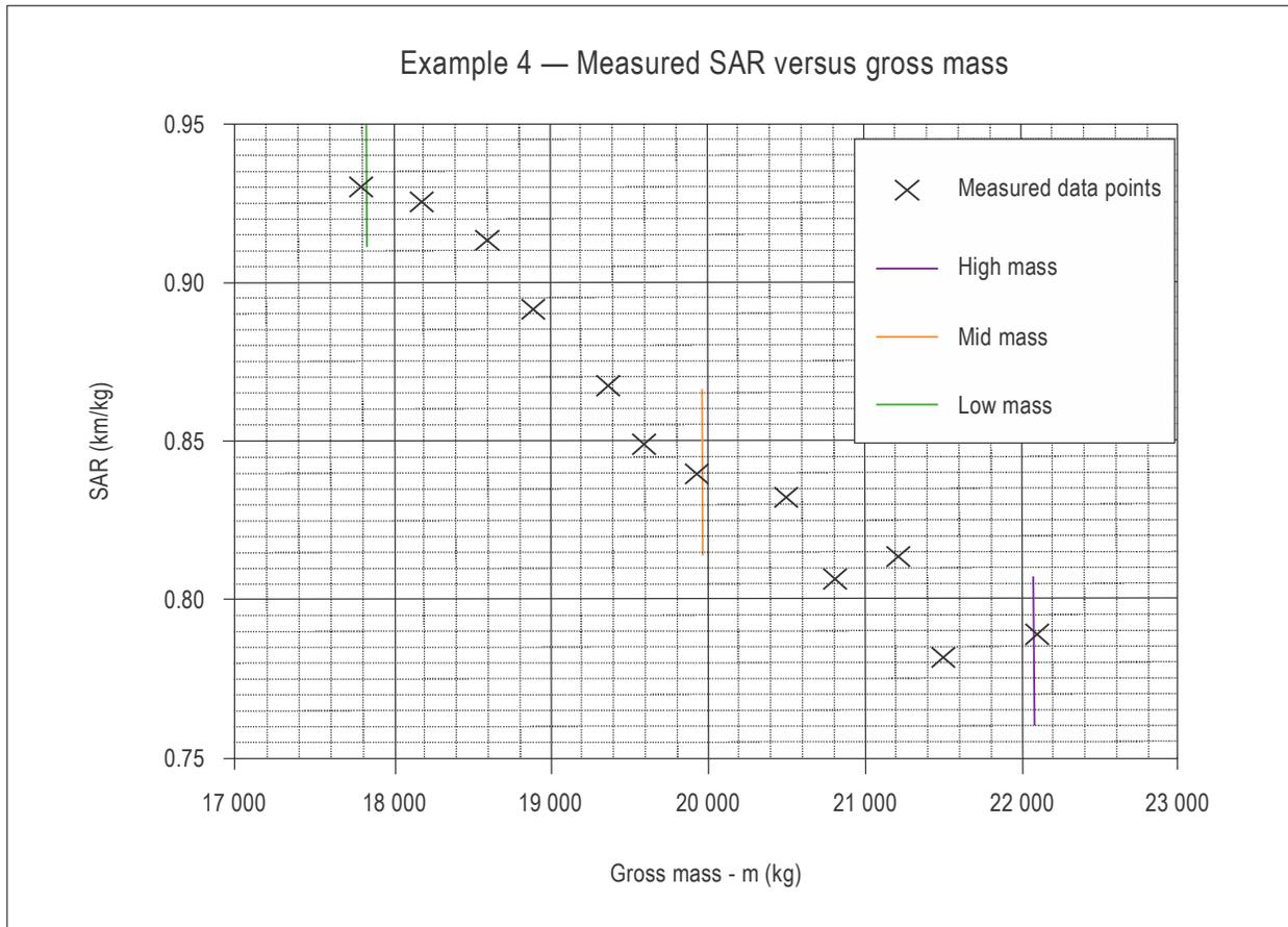
**Figure 3-7. Measured SAR versus gross mass – Example 4**
