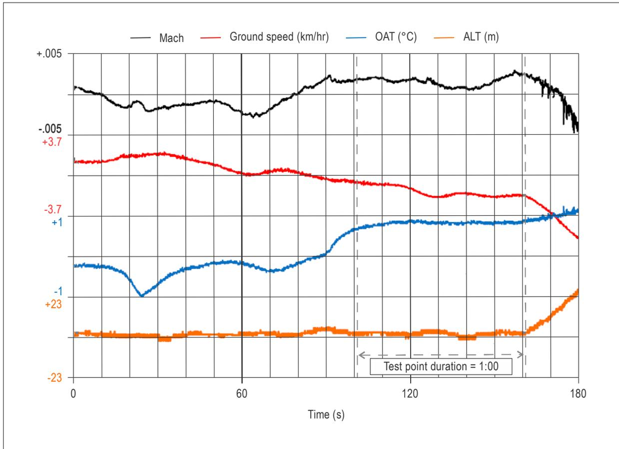
Figure 3-2. Flight test data time interval selection – Example 2
