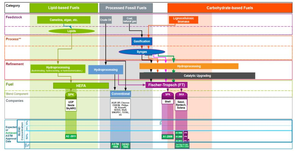
In 2009 the use of other non petroleum feedstocks, i.e. natural gas & biomass using the FT process were permitted to produce SBC and new fuel specification (ASTM **D7566** was created to capture and control the more stringent requirements when producing ATF with SBC. (The SATF-CTL pathway had been an annex in DEF STAN 91-091)
