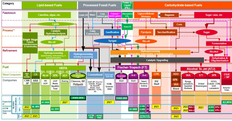
\* Green H = Hydrogen produced from renewable energy sources e.g. wind/solar/hydro \*\* Process / information is shown for diagrammatic purposes only \*\*\* A1, A2, A3, A4, A5, A6, A7 refer to ASTM D7566 annexes \*\*\*\* Dates are estimations only, as of October 2022 Since 2011 the number of SBC pathways in ASTM D7566 has been expanded and the number of approved feedstocks and processes to produce ATF by blending SBC is now seven.
