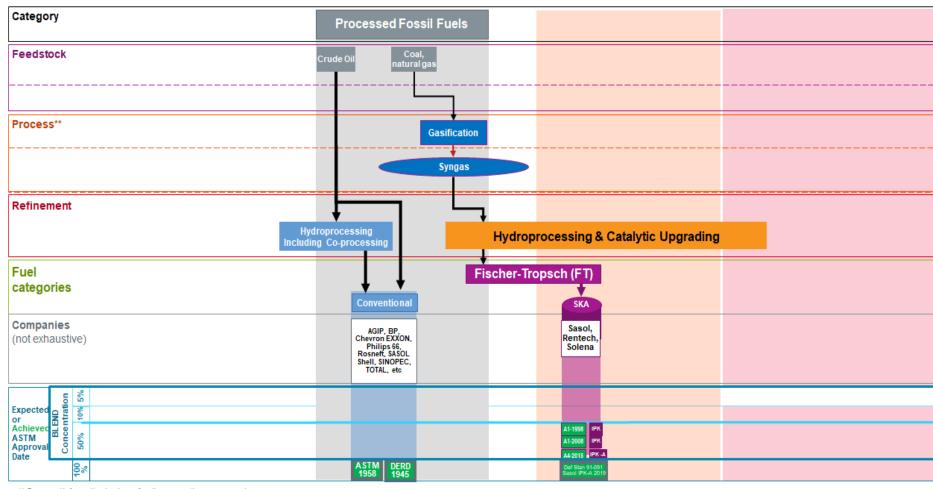
In 1999 the first non petroleum Synthetic **Blending Component** (SBC) production pathway was approved to be used in the production of ATF. **Coal was transformed** using the Fischer **Tropsch (FT) Process &** the SBC was blended with ATF to make the first SATF known as Coal-To-Liquids (CTL). SATF-CTL has been safely used in South Africa for over 20 years
