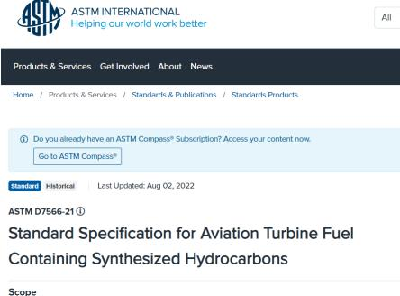
1.1 This specification covers the manufacture of aviation turbine fuel that consists of conventional and synthetic blending components.
