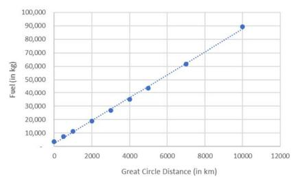
Figure 5: Illustration of generic aeroplane ICAO CEM
