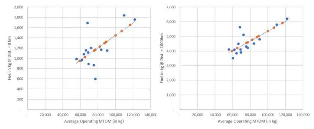
Figure 4: Illustration of generic aeroplane fuel burn-MTOM based regressions for a given distance
