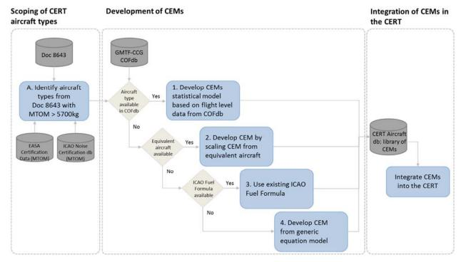
Figure 13: Summary of process for developing ICAO CO<sub>2</sub> Emissions Estimation Models (CEMs)
