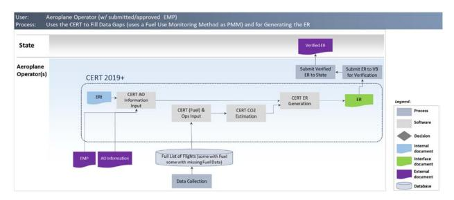
Figure 7: Mapping of processes supported by the 2019+ versions of the ICAO CORSIA CERT for an aeroplane operator with an approved EMP and using the ICAO CORSIA CERT to fill data gaps and generate its ER
