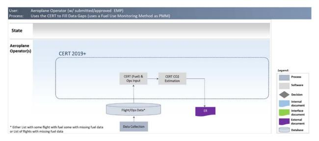
Figure 8: Mapping of processes supported by the 2019+ versions of the ICAO CORSIA CERT for an aeroplane operator using the ICAO CORSIA CERT only to fill data gaps
