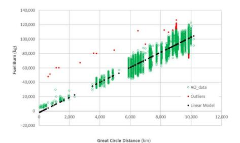
Figure 15: Illustration of sample data used to generate ICAO CEMs, including outlier data removed from the process of generating the ICAO CEM
