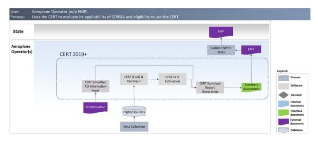
Figure 9: Mapping of processes supported by the 2019+ versions of the ICAO CORSIA CERT for an aeroplane operator to determine the applicability of CORSIA and eligibility to user the ICAO CORSIA CERT
