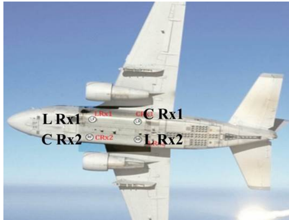
Four receiver (Rx) antennas: 2 in C-band, 2 in L-band
