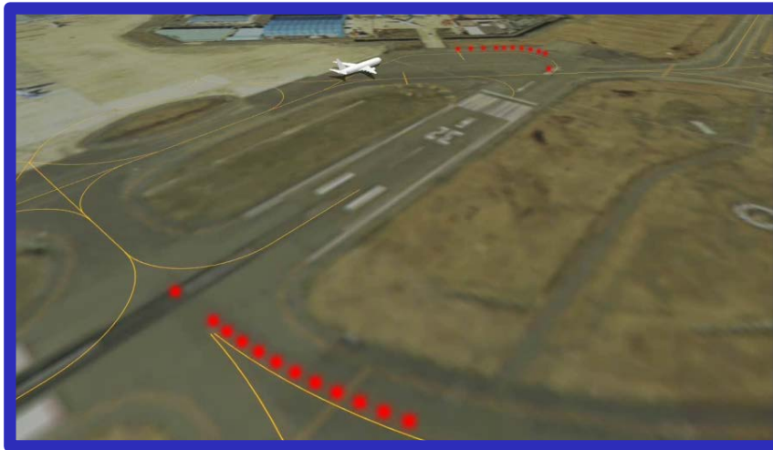
Example of REL and THL (Osaka Int'l: Entering from C1 to take-off from A-RWY)
