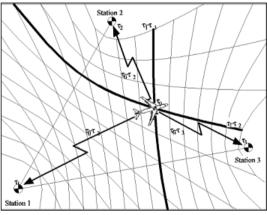
This principle can be extended to measure 3D positions : a 4<sup>th</sup> ground station is then required
