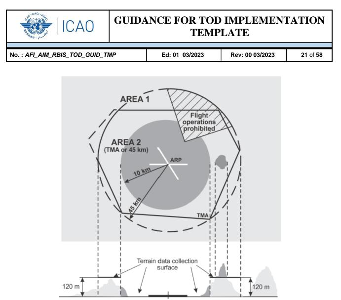
ARP Terrain data collected with Area 1 numerical requirements Terrain data collected with Area 2 numerical requirements Figure 5: Terrain data collection surfaces — Area 1 and Area 2
