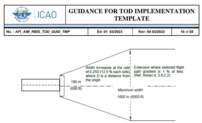
Figure 2: Graphical representation of take-off flight path area as defined in ICAO Annex 4
