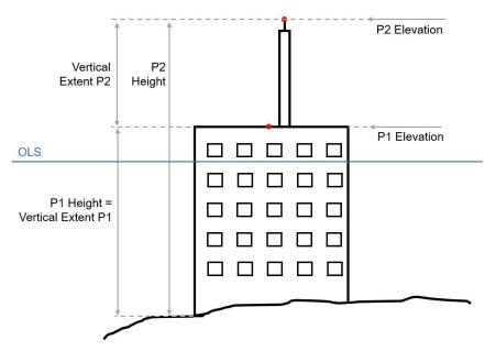
Figure A14: Example of a segmented obstacle
