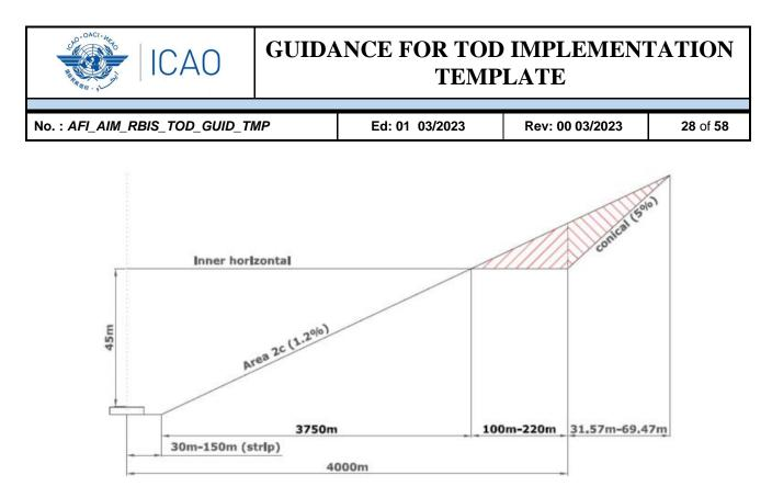
Figure 10: Gaps between Area2c 1.2% Surface and Obstacle Limitation Surfaces
