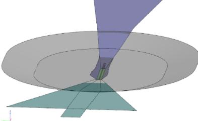
Figure 1: Graphical representation of the listed obstacle limitation surfaces
