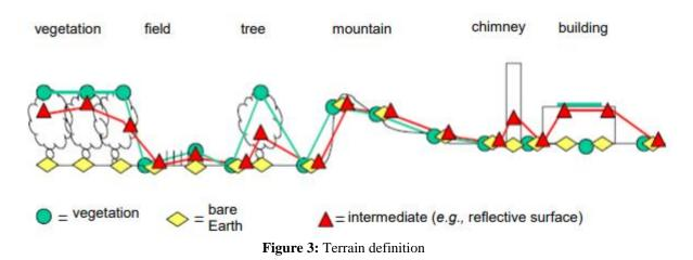
The terrain must be represented by elevation at regular intervals. The result is a digital elevation model.
