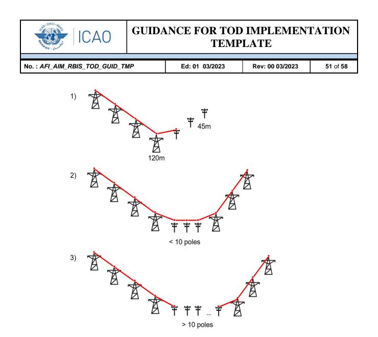
Figure A11: Capture of power lines with segments below the collection surface
