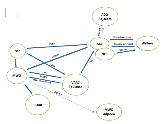
*Figure 2*: Coordination between the entities in accordance with the AFI Volcanic Ash Plan and National Plans.
