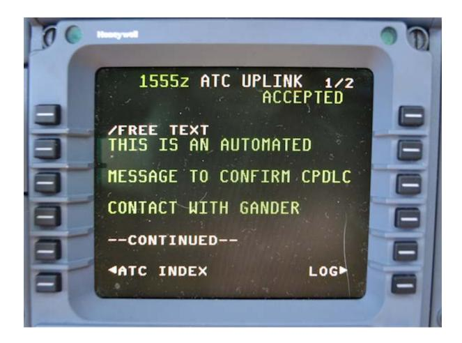
CPDLC provides air-ground data communication for the ATC services.
