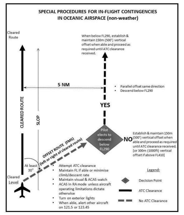
Figure 13-1. Visual aid for understanding and applying the contingency procedures guidance.
