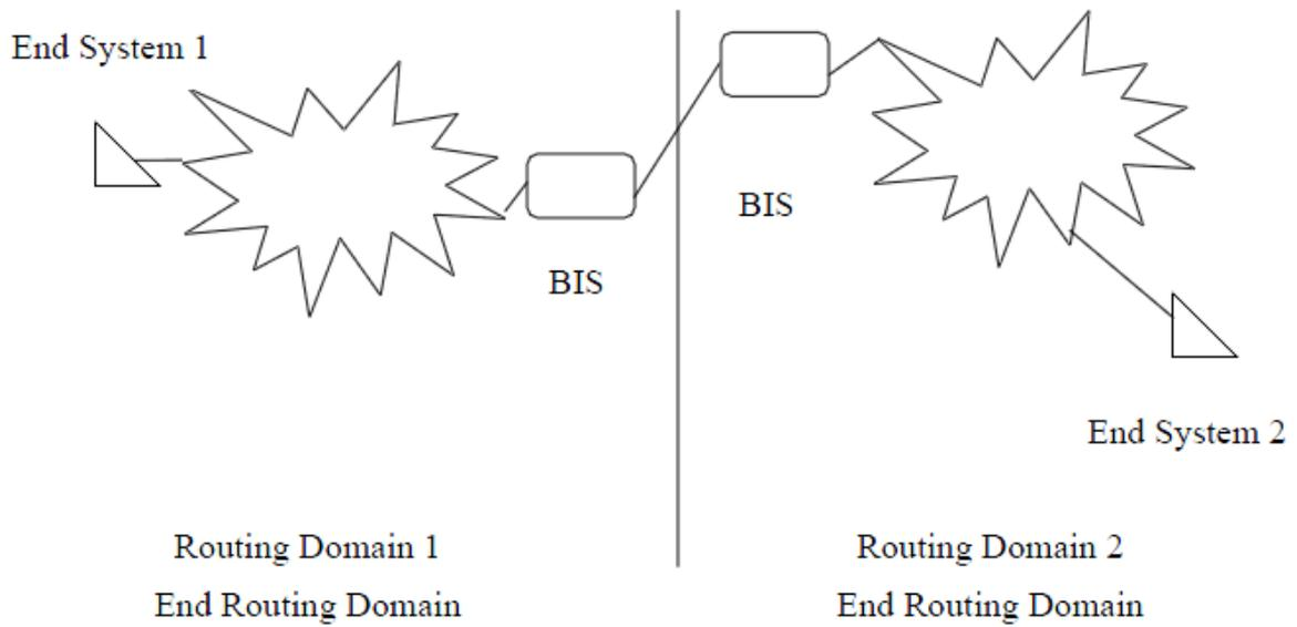
**Figure 1 – End Routing Domains**
