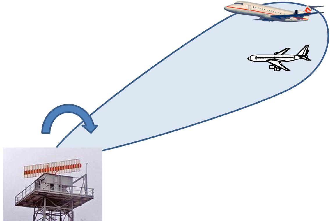
**However, Mode S can do adaptive interrogations. The Stochastic All-call interrogation asks for replies to be sent with a probability of less than 1. Chances are the two A/Cs come up with different probabilities so both don't reply to each interrogation. So both are acquired.**
