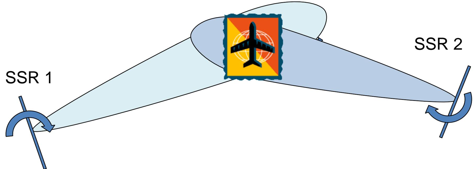
**Adjacent SSRs have the same pulse repetition frequencies (PRFs) – if pulses collide or are too close, the aircraft won't be detected**
