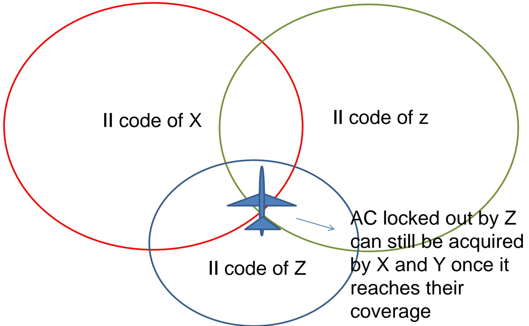
**Examples of how limited II codes (0 to 15) should be used judiciously! For a handful of radars, manual assignment of codes is easier!**
