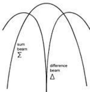
In order to overcome the deficiencies in modes A and C recognized it was proposed a new interrogation format. The new system was intended to operate with just a single reply from an aircraft, a system known as monopulse.
