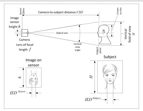
Figure 5 — Illustration of optical arrangement and terminology
