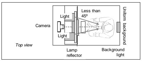
Figure A.7 — Example of a photo booth setup: Top view.
