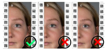
Figure 12 — a) Part of a compliant portrait, b) Image sharp at nose only, c) Image sharp at the ears only.
