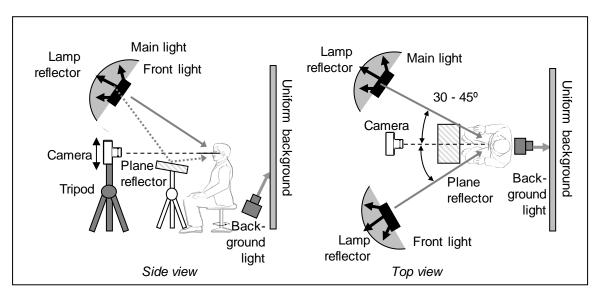
Figure A.3 — Example of a setup with two front lights and one background light
