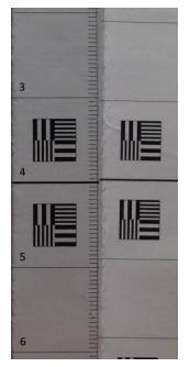
Figure B.6 – Example measurement of the magnification distortion effect.
