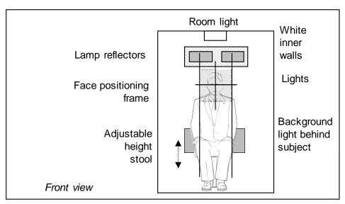
Figure A.4 — Example of a photo booth setup: Front view.
