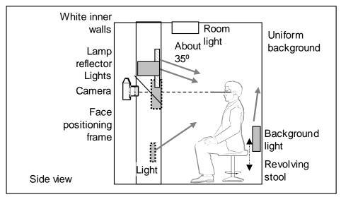
Figure A.5 — Example of a photo booth setup: Side view.
