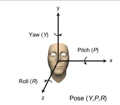
Figure 24 – Definition of pose angles with respect to the frontal view of the subject.
