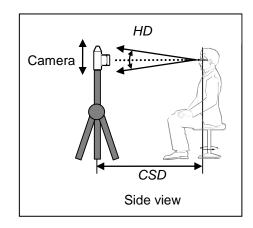
Figure 6 — Alignment of camera and subject
