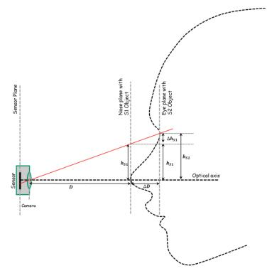
Figure F.1 — Illustration of magnification distortion
