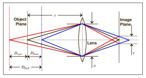
Figure E.1 — Dimensions for depth-of-field calculations
