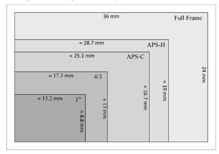
Figure 4 — Typical sensors and their relation in size to the traditional 35 mm full frame
