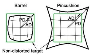
Figure B.9 - Barrel and pincushion distortion
