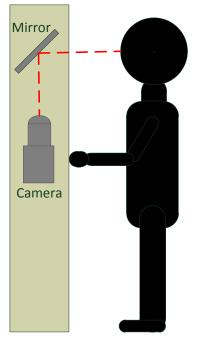
Figure 10 — Principle sketch of a folded optical path.
