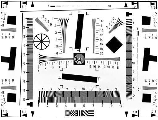
Figure D.3 — Test pattern: ISO 12233:2014.
