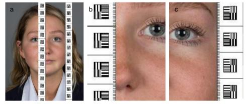
Figure 9 — a) photo captured with rulers at nose and eye level, b) detail showing the millimeter scales at nose level, c) detail showing the millimeter scales at eye level.
