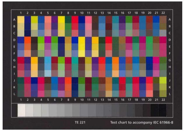
Figure C.1 — IEC 61966-8 colour test chart.
