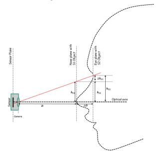
Figure B.5 – Illustration of the magnification distortion effect.
