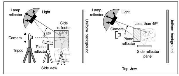
Figure A.1 — Example of a setup with one single light
