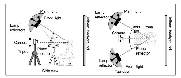
Figure A.2 — Example of a setup with two front lights
