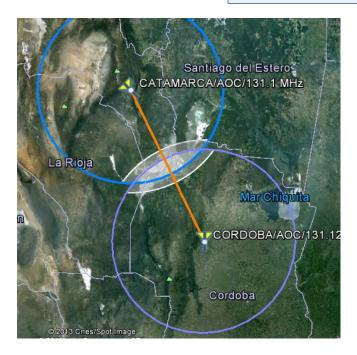
Adjacent frequency interference shows as a circle-se3gment with a buffer zone of 10 NM outside the coverage of the interferer.
