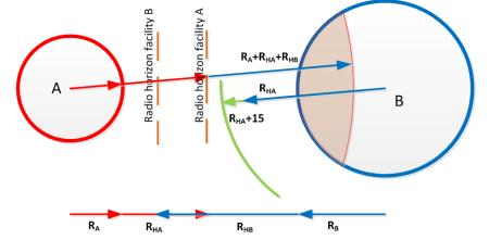
Figure H-13 Interference mechanism between broadcast services; interference contours
