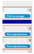
For each frequency assignment that has been tested the button "Plot interference" has been placed. This button permits the user to plot a single interference case on the map. This facilitates the analysis of interference cases when using the map. In case no interference has been calculated (and for the first frequency assignment on the list) the button plots only the designated coverage on the map. The numbered field indicates the order of the records in the table.
