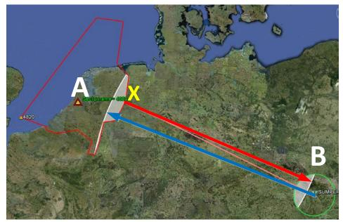
Figure H-8 Interference between facilities with a circular DOC and an area DOC as is presented with Frequency Finder
