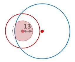
Figure H-19 Interference contour/area when the minimum separation distance requirements between broadcast services operating on adjacent frequencies are not satisfied.
