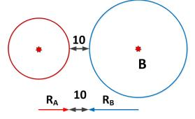
Figure H-15 Minimum separation between circular facilities operating on adjacent frequencies
