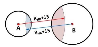
Figure H-11 Interference mechanism between broadcast services
