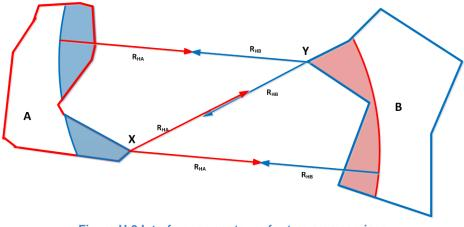
Figure H-9 Interference contours for two area services
