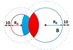
Figure H-16 Interference contours/areas between circular facilities operating on adjacent frequencies
