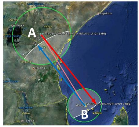
Figure H-6 Interference between two facilities with a circular DOC as presented with Frequency Finder
