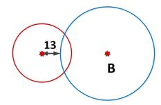
Figure H-18 Minimum separation distance between broadcast services operating on adjacent frequencies
