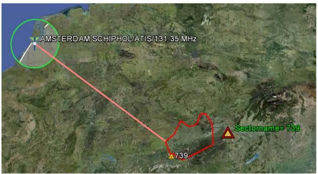
Figure H-13 Presentation of interference between an (area) air/ground service and a broadcast service in Frequency Finder
