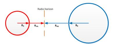
Figure H-4 Separation based on radio line-of-sight as in Figure H-1; seen from above
