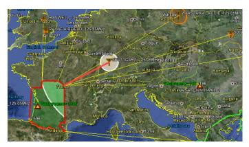
Co-frequency interference between Bordeaux-ACC (area service) and Stuttgart APP; the interfered stations are connected with a red line; station that do not interfere with each other are connected with a thin yellow line.
