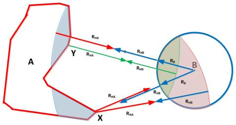
Figure H-7 Interference contours for one area service and one circular service
