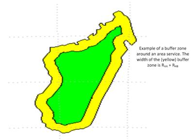
Figure H-2 Example of buffer zone (interference contour) for an area service (e.g. FIS)
