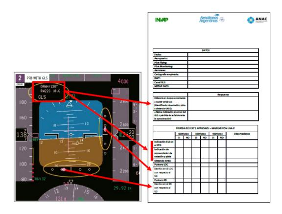
4.7 Thus, on 28 June 2018, for the first time in Argentina, a CAT I approach was performed to threshold 29 of the San Carlos de Bariloche airport, receiving GLS information from the GBAS station installed therein. Images obtained in the PFD (Primary Flight Display) are shown below.
