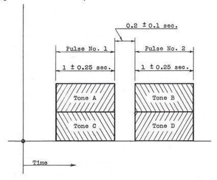
A special decoder on the aircraft's radio is programmed to recognize only the audio frequencies of the SELCAL code assigned to the aircraft. When the decoder receives the correct aircraft SELCAL code, the decoder sends an alert message to the crew, so they can turn the radio audio volume back up to talk with the ground station radio operator.
