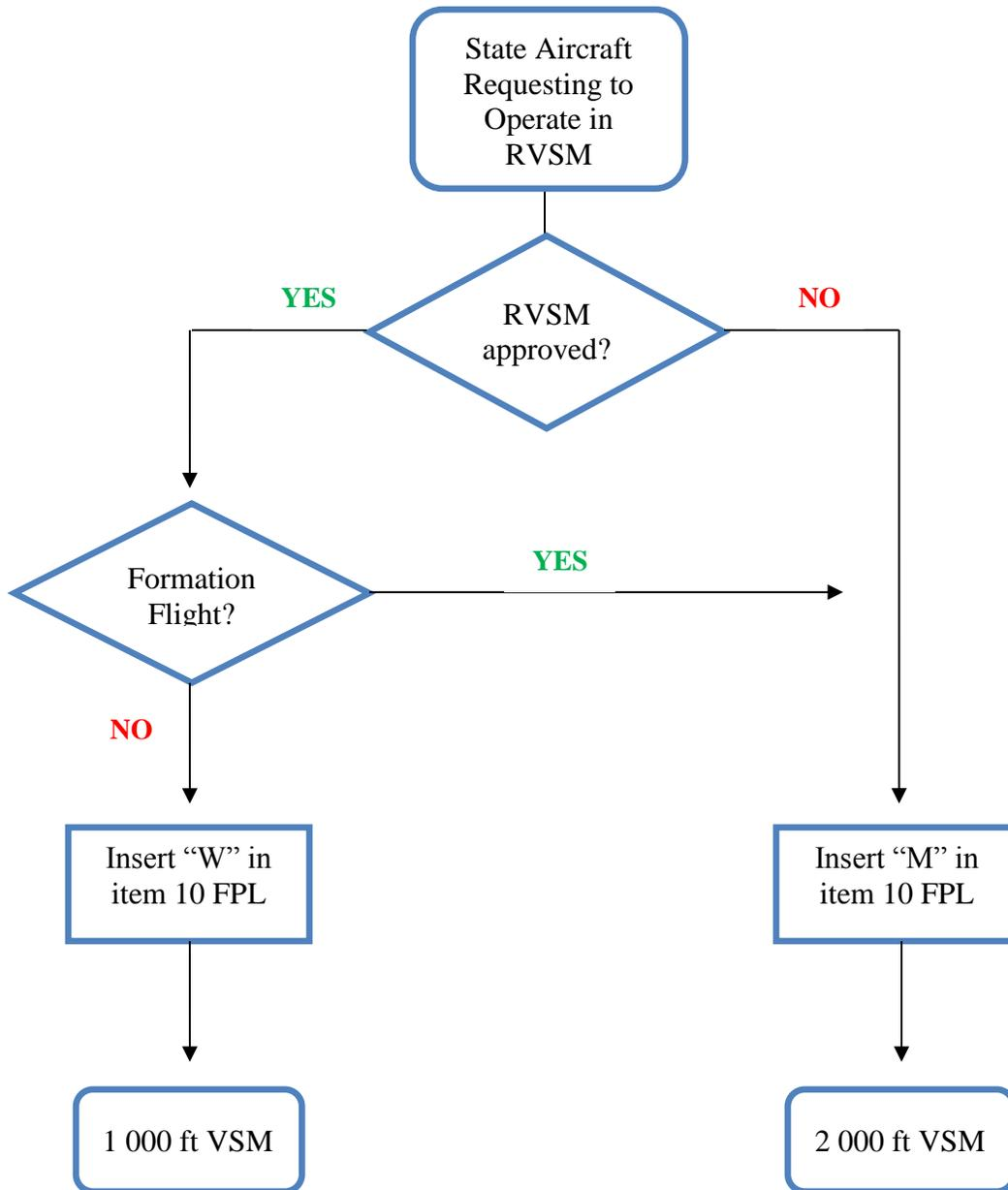
**Figure 2: Flight planning requirements for State aircraft in RVSM airspace**
