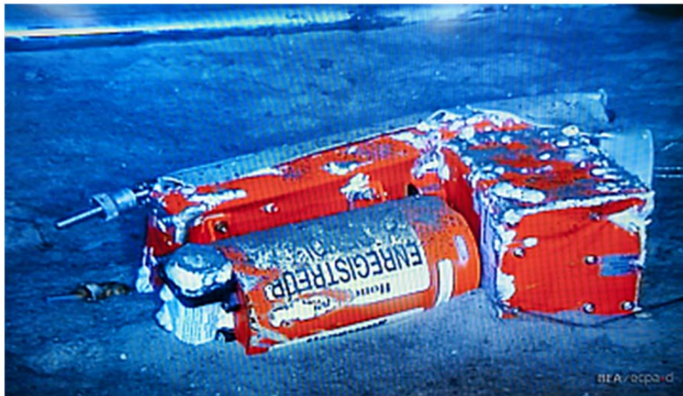
Figure I-5-5. The flight data recorder (FDR) of an Airbus A330 photographed at a depth of 3 900 m in the Atlantic Ocean (2009 accident)
