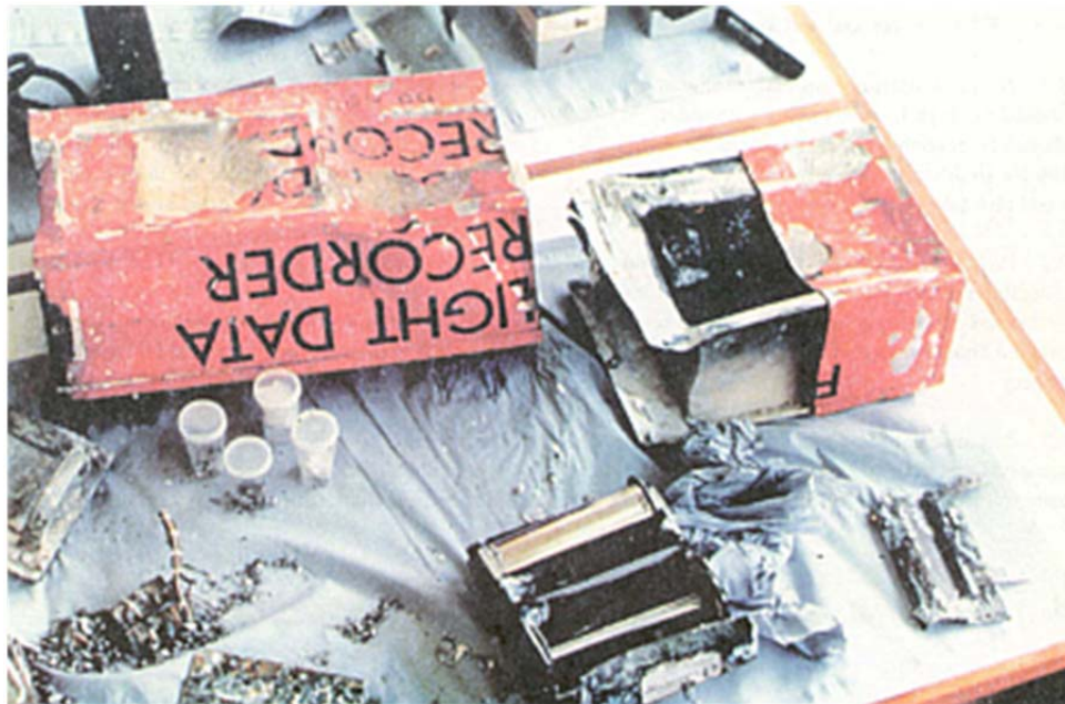
Figure I-5-10. The FDR of a DC-9 showed little corrosion after being submerged for 12 years in the Mediterranean Sea (1980 accident)
