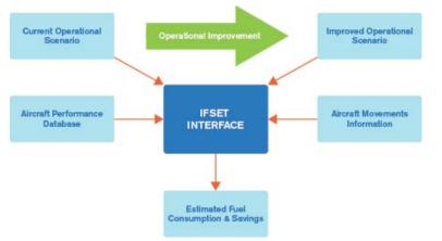
Current Operational Scenario Operational Improvement Improved Operational Scenario Aircraft Performance Database IFSET INTERFACE Aircraft Movements Information Estimated Fuel Consumption & Savings
