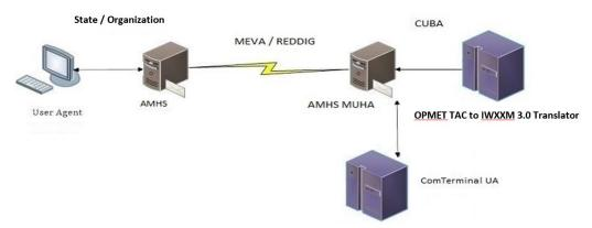
Fig. 1: Test environment for OPMET data exchange according to IWXXM.
