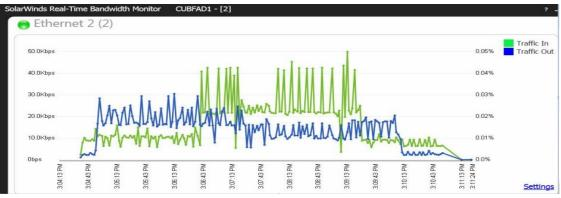
Fig. 2: Bandwidth utilization during a load stress procedure between Cuba and United States.
