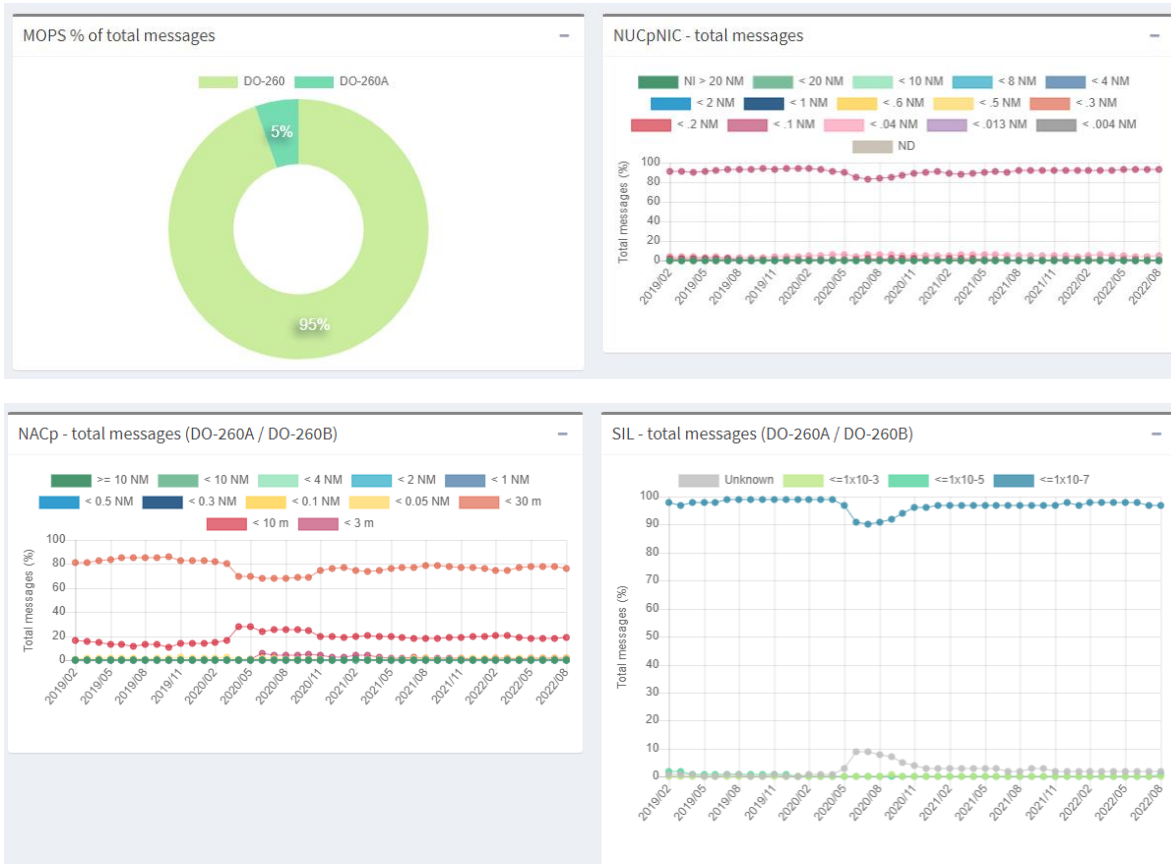
Fig. 4.- Statistics of the main ADS-B figures of merit
