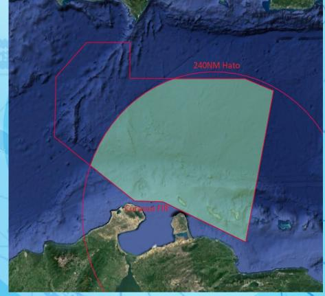
Surveillance coverage within the TNCF FIR based on Hato radar coverage without ADSB-space based
