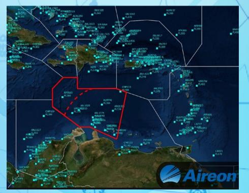
Surveillance coverage within the Curaçao FIR based on Hato radar and Space Based ADSB
