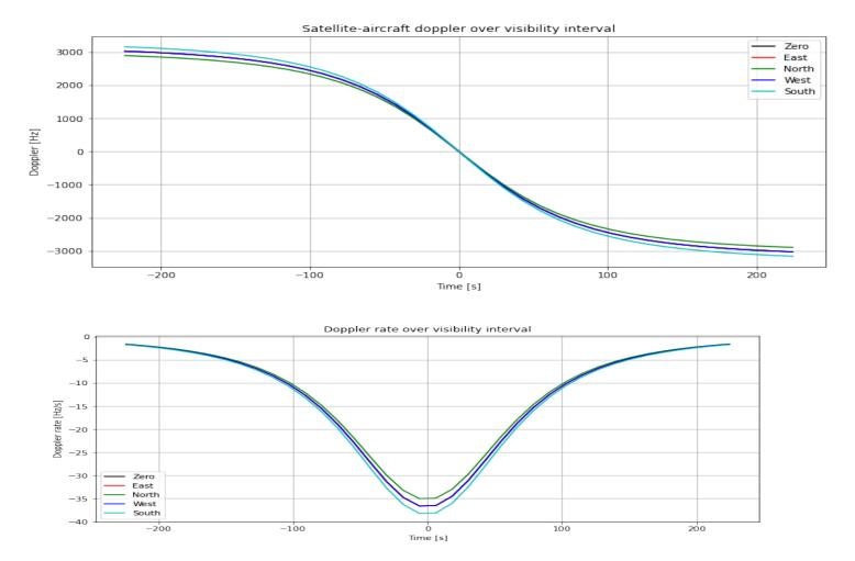
Doppler shift and Doppler rate experienced by an aircraft as function of time in a spacecraft overflight when flying from North to South
