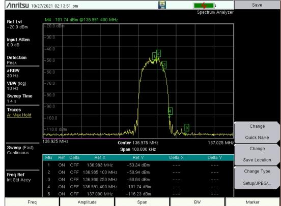
Out of Band (OoB) power at 137 MHz is attenuated higher than 60
