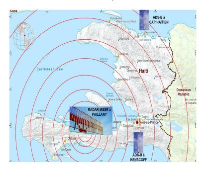
2.4 This Surveillance system gives the final coverage displayed below at FL300 and we are looking to enhance its integrity for our operational needs by implementing Radar Data sharing with our adjacent FIRs like Dominican Republic, Cuba, Jamaica, and the FAA regarding the Grand Turk radar. We've already initiated the talk and all of them have responded positively to our request.
