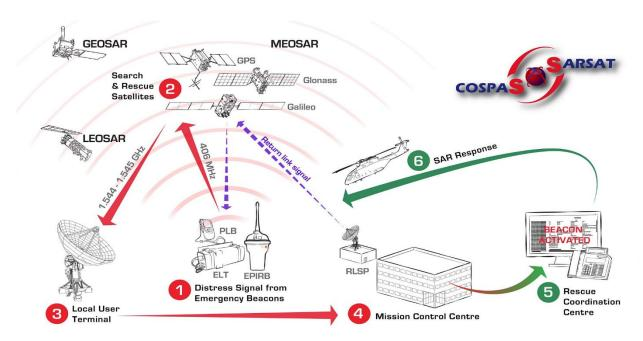
Figure 6: The Cospas-Sarsat system concept, including the new Return Link Service
