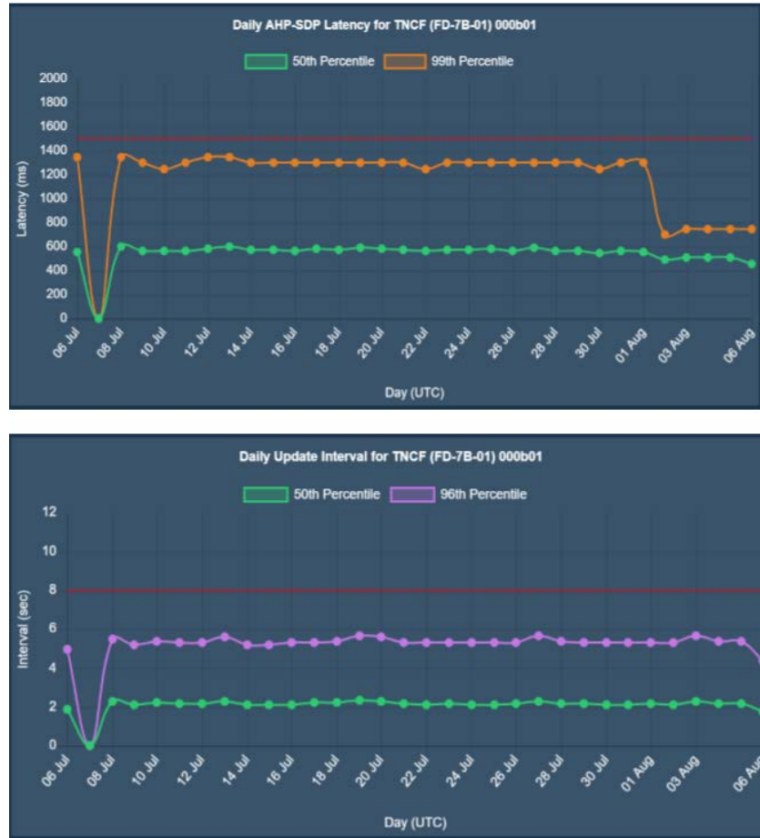
Figure 5. Latency and Update Interval with the use of MEVA at DC-ANSP
