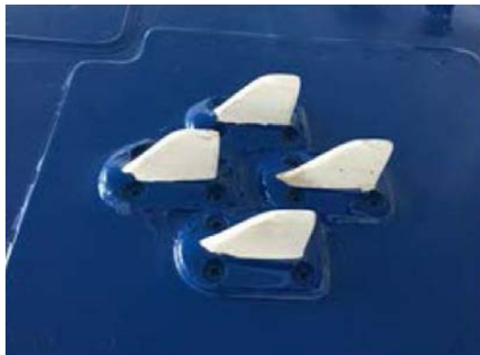
Aircraft bottom mounted direction-finding array (multiple frequency bands), French Flight Inspection
