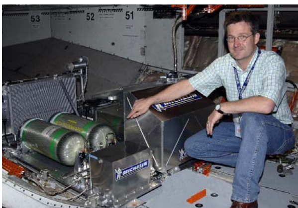
Fuel cell equipment for the A320 test aircraft from DLR in February 2008
