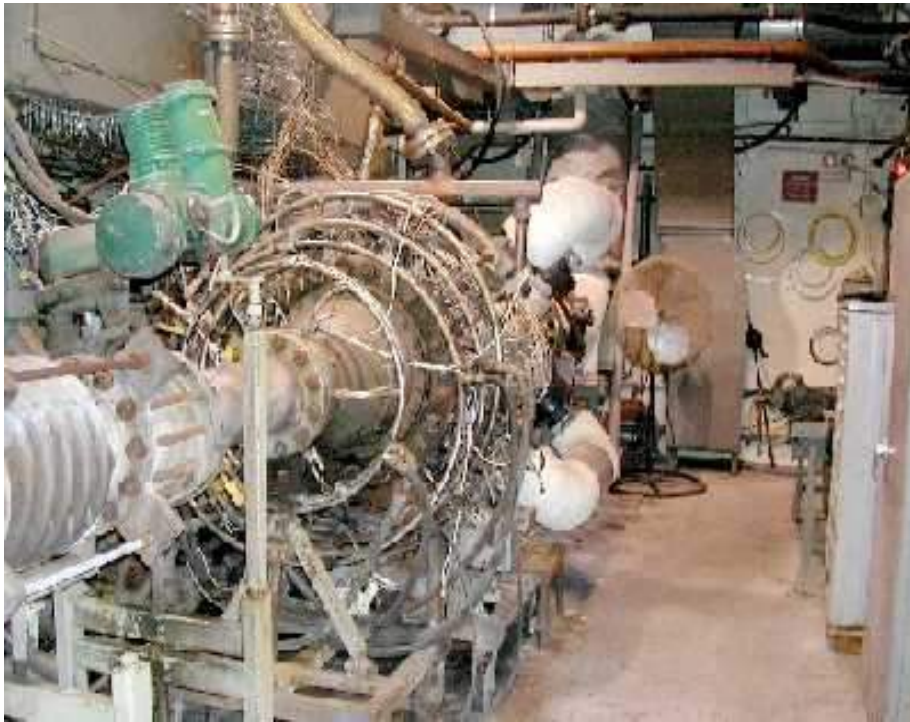
Figure 5: A schematic of the annular rig at Rolls Royce used for testing Alternative fuels.
