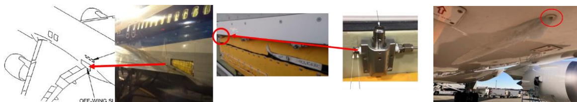
Example of preventive measures (Replacement with improved locking/Cleaning of draining valves)
