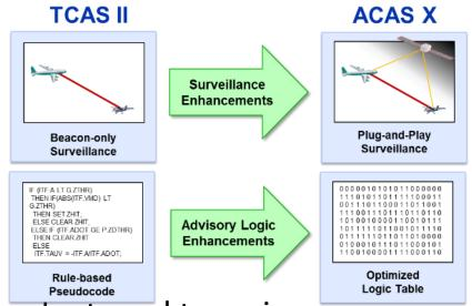
Optimization of resolutions through tools that can be tuned to various sensors and aircraft performance
