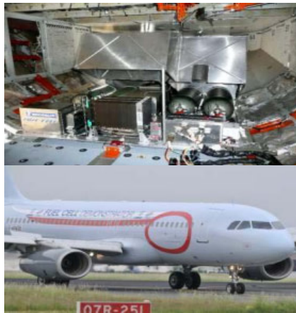
2008: First Functional integration of a fuel cell system. Flight test on A320.
