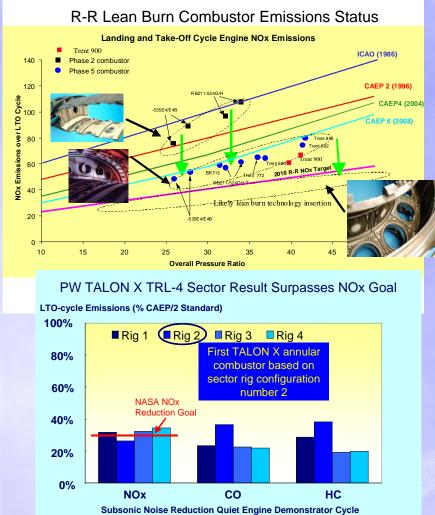
Prototype tests of revolutionary RQL and Lean Staged combustors show potential for considerable NOx reduction
