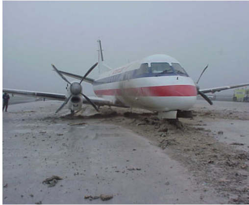
Figure 5 - Photos of EMAS off Runway 22L at JFK taken the day after the safe arrestment of a SAAB-340 overrun in June 1999 (note the surface area removed to extract the aircraft)
