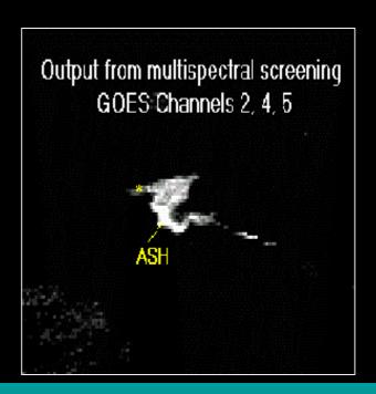
Split Window (left) and the combined image of original and short wavelength infrared images (right) of the GOES satellite. The volcanic ash cloud of Soufriere hills volcano eruption on November 6, 1997 was detected clearer on the latter. (from Gary P. Ellrod (NOAA/NESDIS) et al., 1999).
