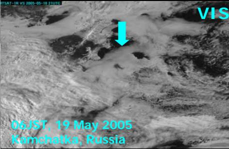
The boundary of fog near Kamchatka is clear in IR4 channel at night, while not in the existing IR1 ch
