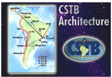
3.2 The TMS collects all TRS data and determines the amount of error associated with the GPS system in each respective geographic region represented by each TRS. This correction data is then formatted for broadcast and forwarded to either a VHF broadcast tower or Geostationary Communications Satellite (GEO) if available for transmission to the users.
