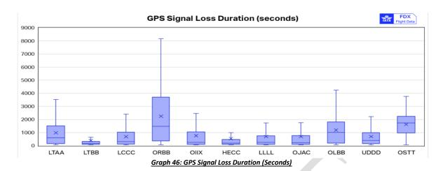
Sorting by average seconds of GPS Signal Lost duration in descending order, ORBB (Baghdad FIR) had the longest duration, in average of 2,251 seconds, followed by OLBB (Beirut FIR) with 1,184 seconds, LTAA (Ankara FIR) with 984 seconds, OIIX (Tehran FIR) with 760 seconds, OJAC (Amman FIR) with 699 seconds, LLLL (Tel-Aviv FIR) with 697 seconds, UDDD (Yerevan FIR) with 691 seconds, LCCC (Nicosia FIR) with 687 seconds, HECC (Cairo FIR) with 536 seconds and LTBB (Istanbul FIR) with 402 seconds.
