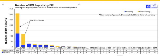
Graph 44: Distribution of GNSS/GPS Interference by FIR
