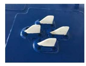
Aircraft bottom mounted direction-finding array (multiple frequency bands), French Flight Inspection
